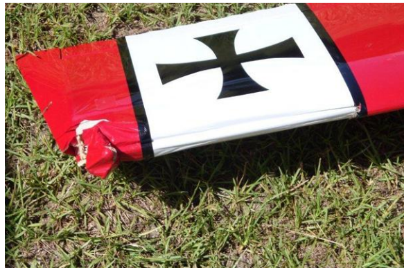
The damage to Terry's Stick. Lesson learned: Plug in connectors correctly and test!
